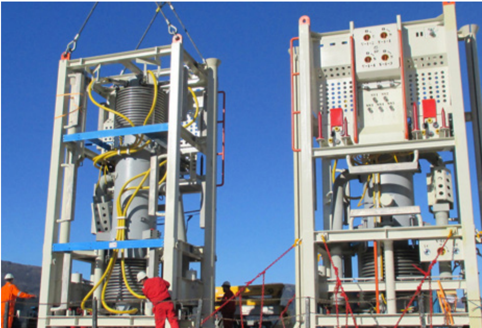
The subsea compression system from OneSubsea is the first and only true subsea wet gas compressor.
