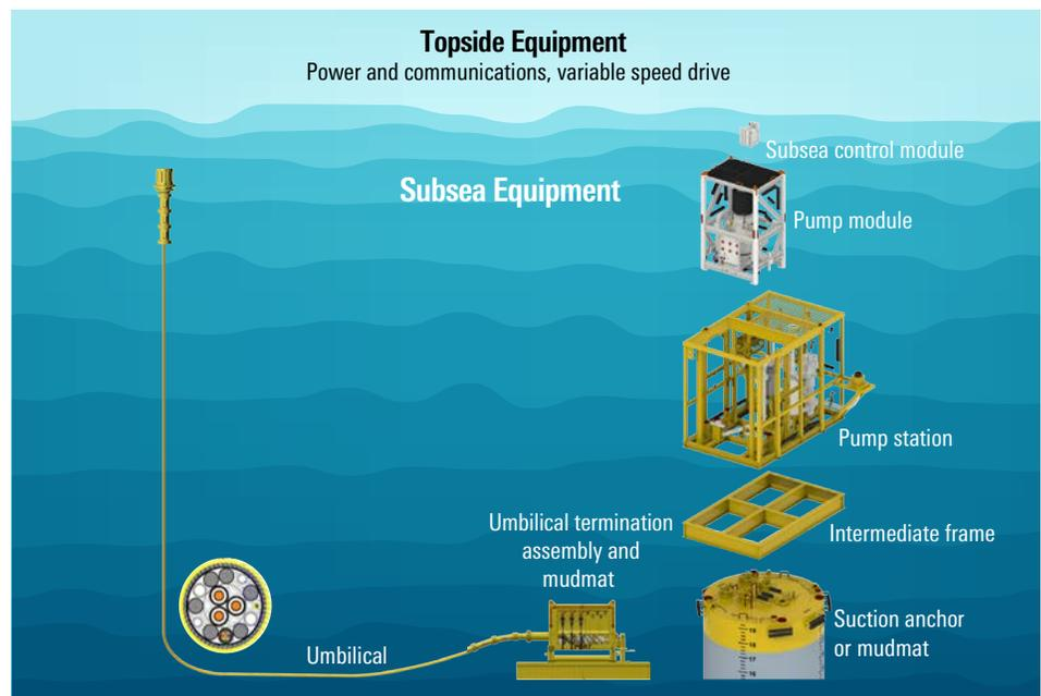
Subsea and topside equipment for OneSubsea boosting systems.
