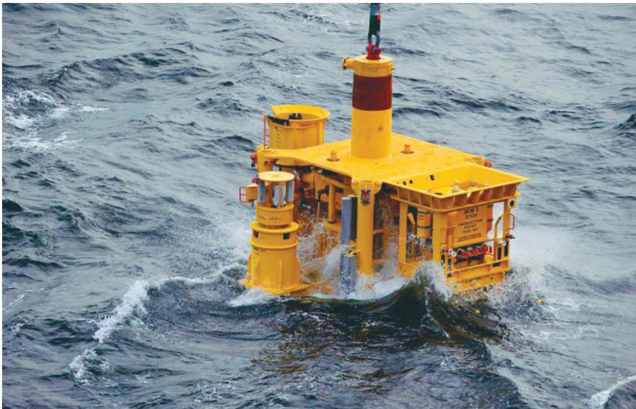
A subsea tree comprised of cost-efficient equipment components. (Source: Schlumberger)
