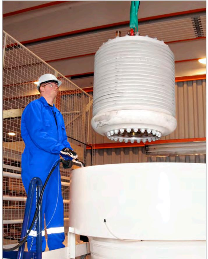
*At the OneSubsea facility in Horsøy, Norway, PhaseWatcher flowmeters undergo rigorous testing at pressures exceeding the expected pressure on the seabed.*
