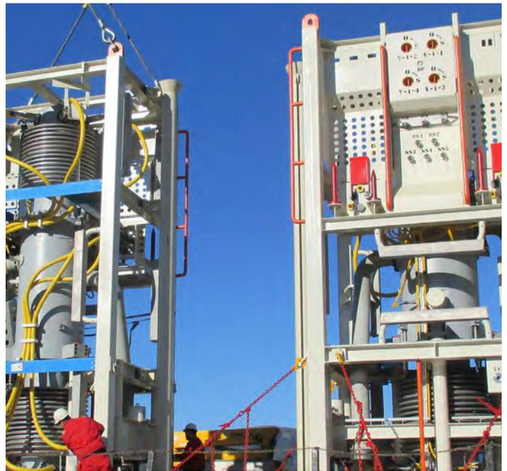
*Two 5-MW rated WGC4000 multiphase compressors.*
