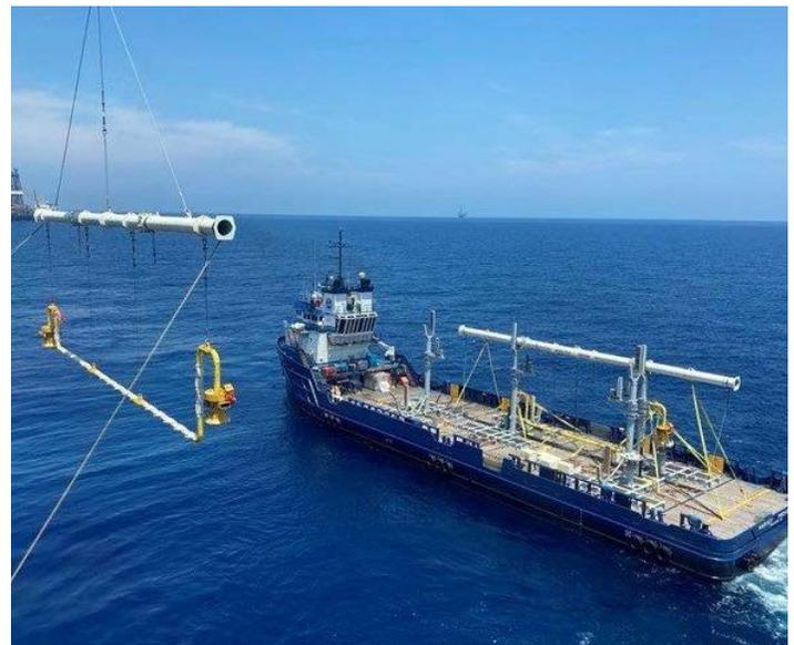
*Subsea jumpers deployed for the Mad Dog Phase 2 project are fitted with an OCS-V clamp connection system (yellow) at each end.*
