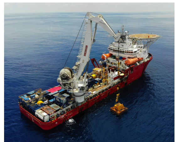
The integrated deepwater intervention campaign included the OneSubsea SMIS, which can be operated from a modest vessel of opportunity rather than from a rig, enabling flexible, streamlined fluid intervention.
