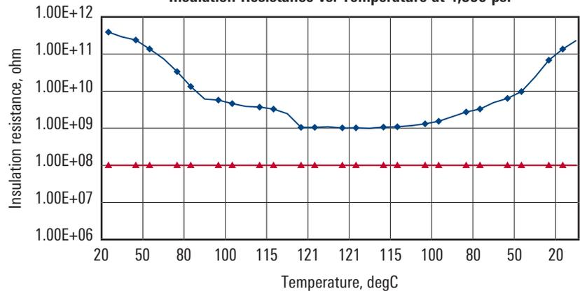
—◆— Connector pair pin to earth    —▲— Pass mark (100,000,000 ohm)
