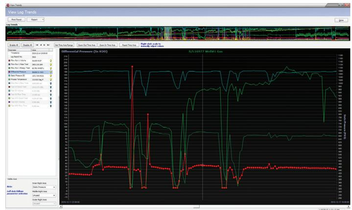
Data may be transferred from the Scanner 3100 flow computer to the PC by an Ethernet connection to a PC operating an FTP client or a browser application. In addition, WiFi, cellular communication, or other wireless methods can support remote data collection.
