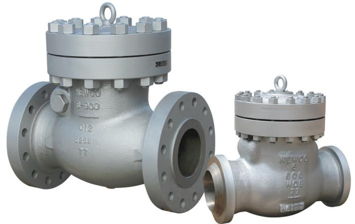
*Ideal for standard and critical power industry applications, NEWCO\* gate, globe, and check valves include a pressure-seal bonnet joint that eliminates the body and bonnet flanges, reducing weight and simplifying the application of exterior insulation.*
